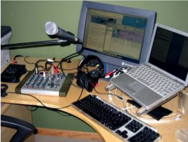
This podcasting setup includes a simple audio mixer, recorder and a computer for recording Skype interviews.
