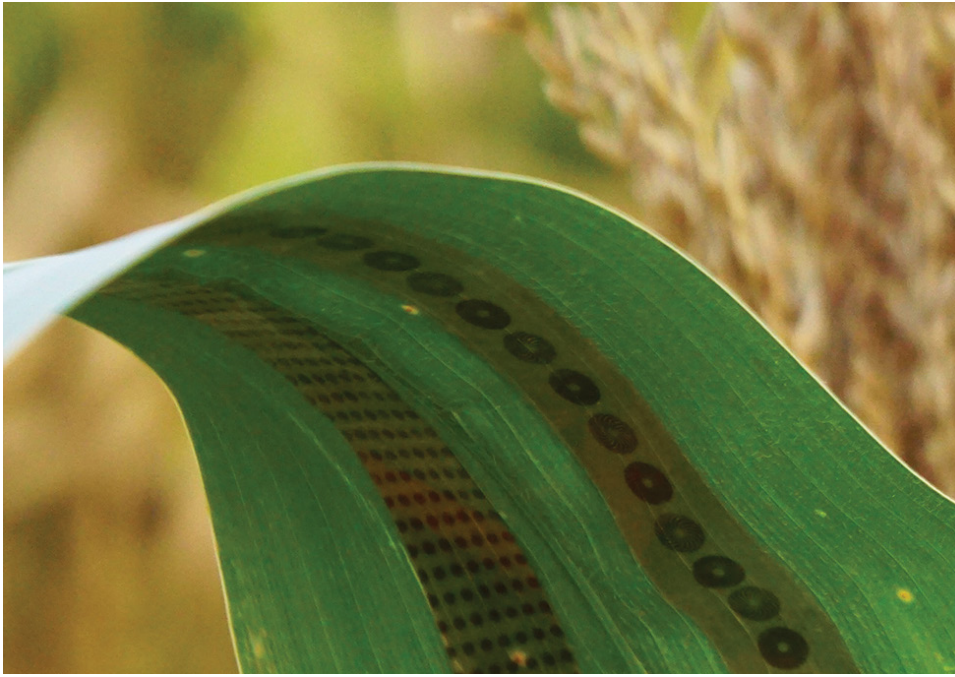
FIGURE 1-7. Small graphene sensors placed on plant leaves are used to sense water transpiration and measure plant water use so that irrigation is only applied when needed.
